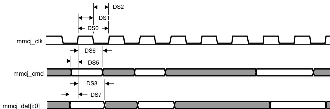
Figure 5-94. MMC/SD/SDIOj in - Default Speed - Receiver Mode
