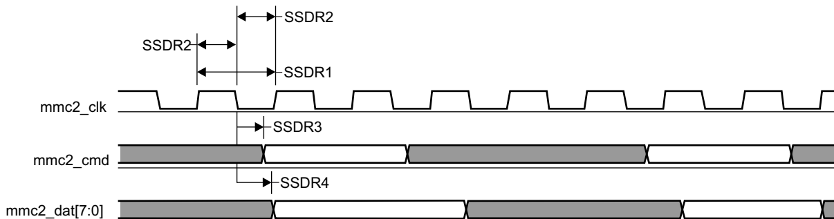
Figure 5-88. MMC/SD/SDIO in - Standard JC64 - Transmitter Mode
