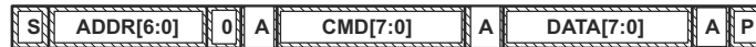
Figure 7-2. Attempt To Write a Read-Only Address (Nack After Data Sent By Master)
